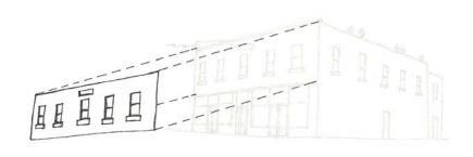
The upper façade consists of any area or floors of the building above the storefront level and below the cornice, including the second floor windows.
