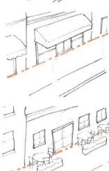
Awning: An awning provides pedestrian shade and protection as it overhangs the sidewalk. It is an encroachment that is allowed due to its public benefit.
