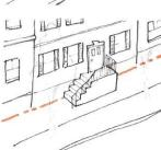
Stoop: This frontage type provides a compact way to access housing when there is no front yard and the entrance floor is above sidewalk level. Stairs run parallel to the street, rather than impeding pedestrian flow.
