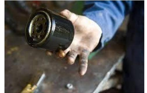
Non-terne used oil filters should be **hot drained** into a properly labeled container *for at least 12 hours*. Once the oil filter is properly drained, the filter can be disposed of as a solid waste along with the other regular trash in your solid waste dumpster. If you choose not to hot drain the filters, then the filters should be managed as used oil.
